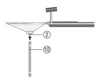
The corrugated tube (10) that is included in the scope of supply is pushed onto the discharge nozzle (2) of the Collecting Bag.
