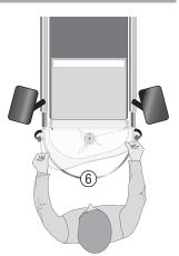
The rounded bag edge is fitted over the spring brace (6) and the holding rod is inserted into the spring brace holders.
