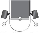
The holding rod (3) is removed at the spring brace holders (4).
