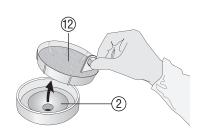
The filter sieve (10) holds back tissue fragments and thus prevents the conduit from becoming blocked. It can be removed from the discharge nozzle (2).
