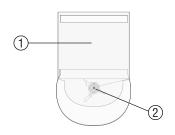
The TUR Collecting Bag (1) is unfolded. The discharge nozzle (2) points downwards (see also illustration 8).
